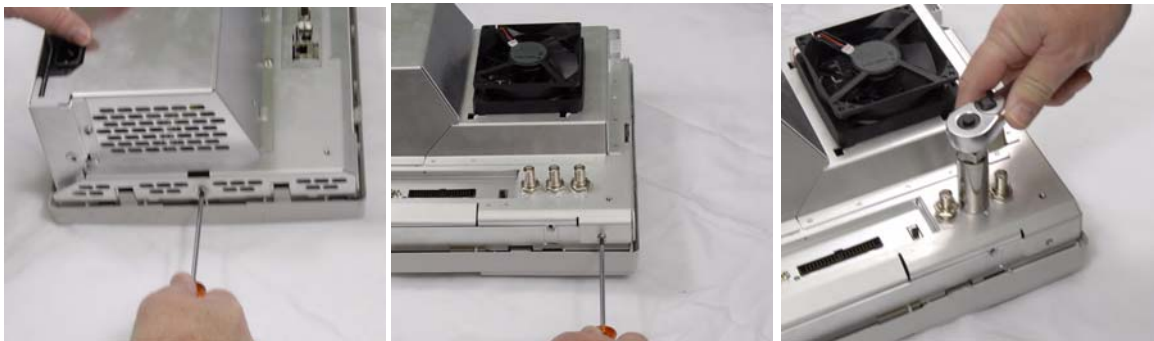
Figure 19 Removing the rear deck assembly
