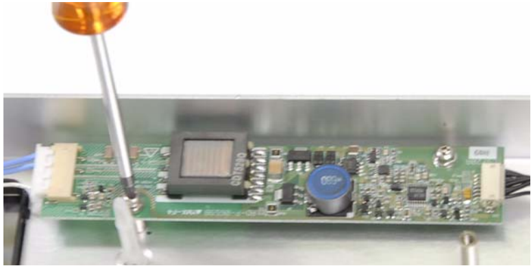
Figure 24 Removal of inverter board
