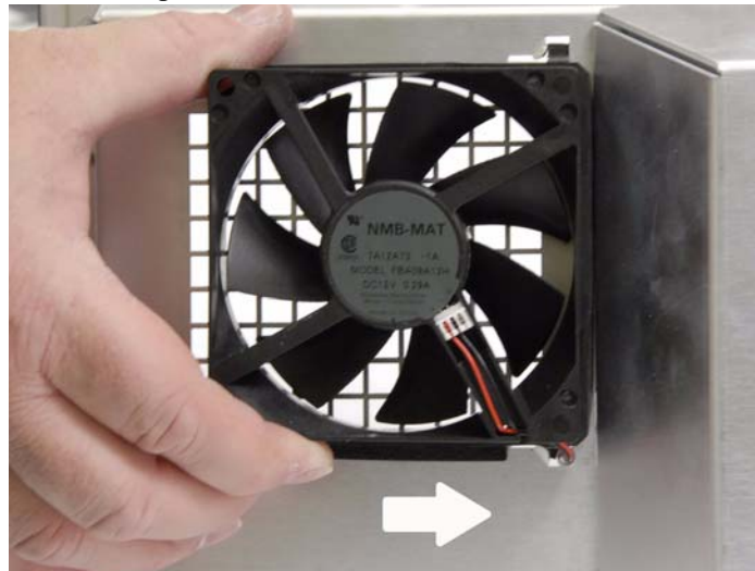
Figure 35 Removing fan assembly
