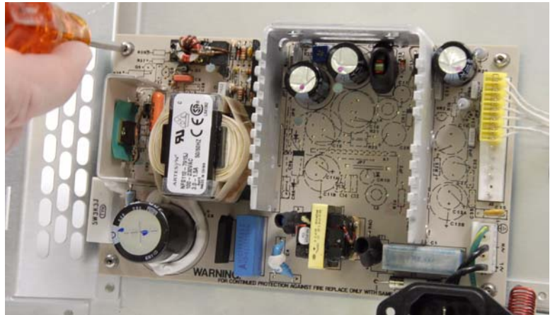
Figure 38 Removing the power supply
